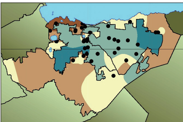
Soil classification map based on Vs-20 analysis of Managua. The black points represent the investigated points and the color indicate the average shear velocity of the soil.
