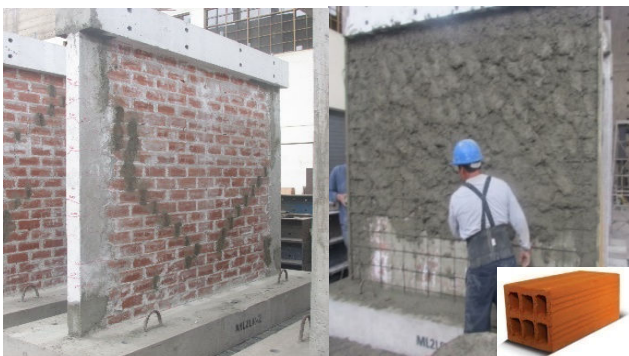
Fig. 1. Original walls of masonry (left), wall retrofitting with steel mesh (right), coating with mortar cement-sand, unit of Pandereta brick (lower right).
