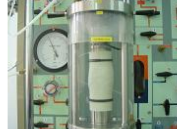
Shear failure of tested sample
