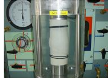
Shear failure of tested sample
