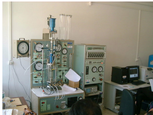
Fig. 1 Triaxial Testing Apparatus Model DTC-367 by Seiken.Inc. Japan (Photo at NCSRR)
